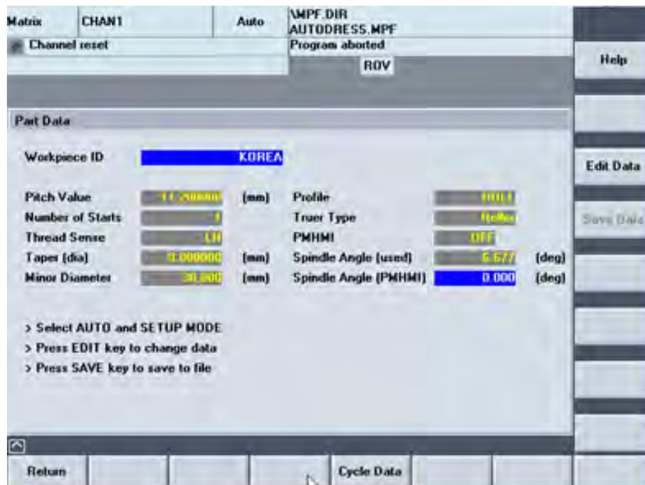
Before proceeding to grind a workpiece thread you **must** enter part data about the workpiece to be ground.
