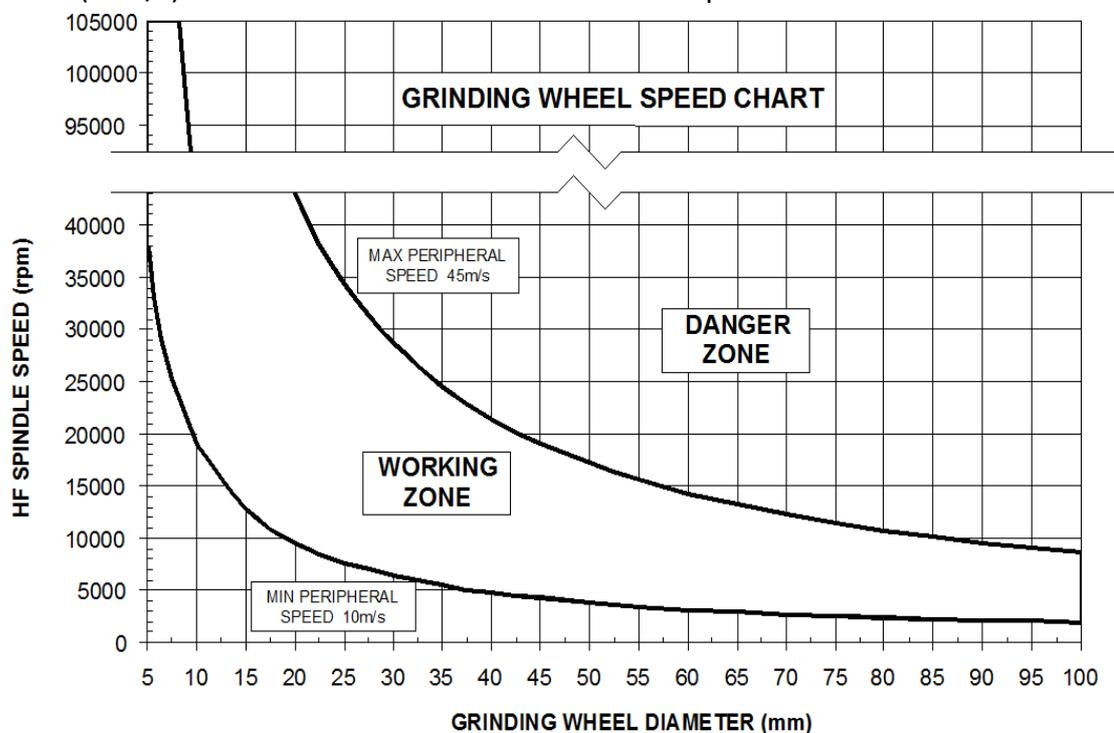
Every effort should be made to ensure that the grinding wheel speed operates within the “Working Zone” shown on the chart.
