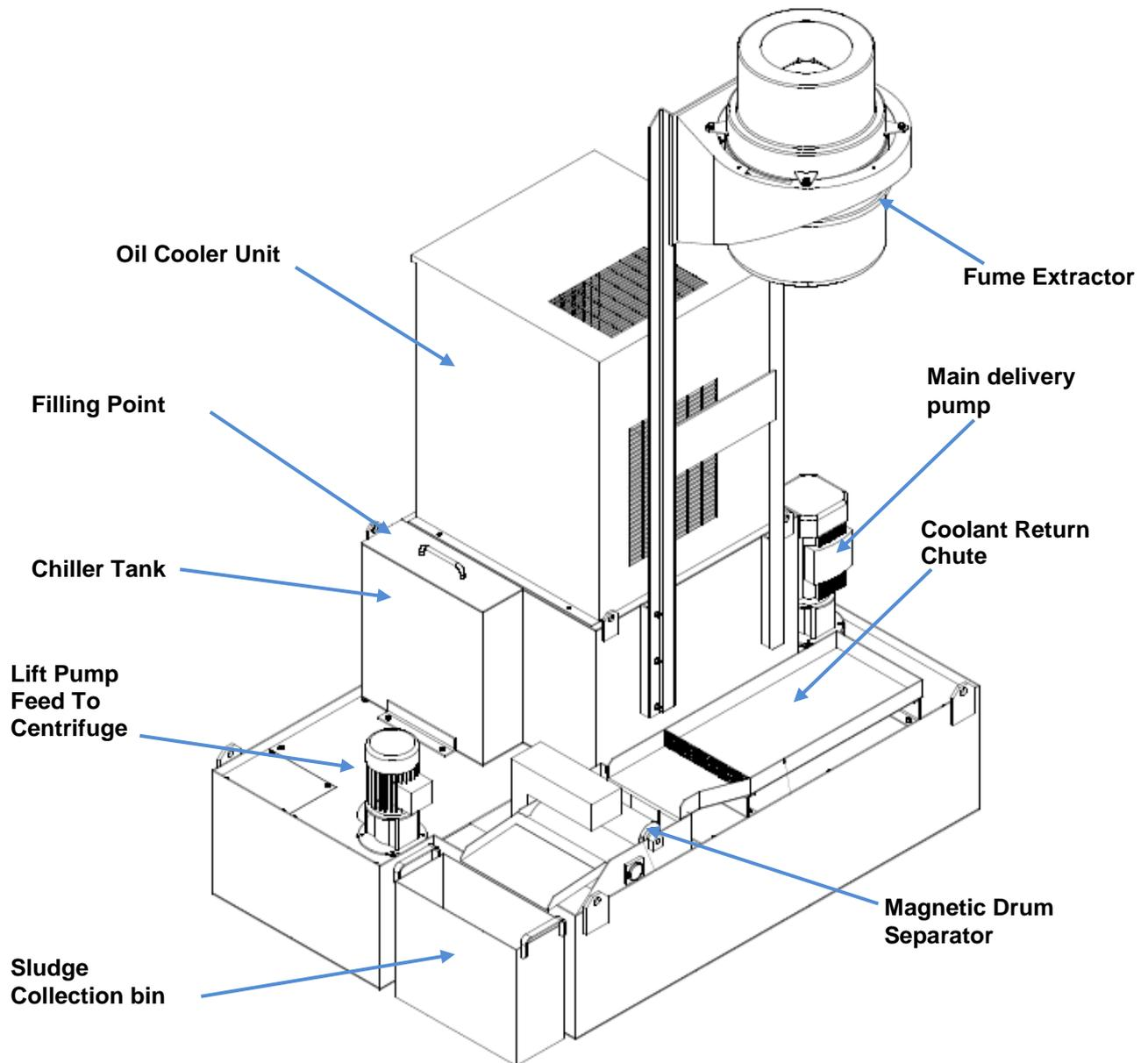
Fig.33.0a —Coolant Clarifier System.
