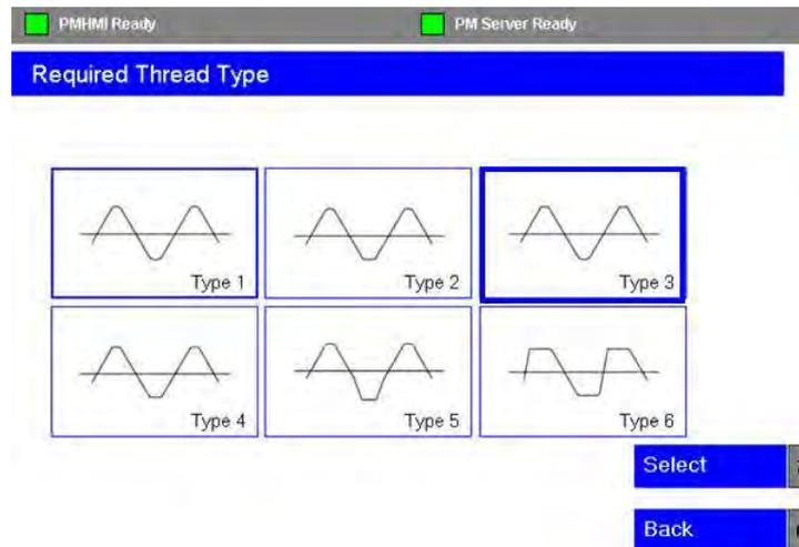
1. Highlight the Type 3 icon using the blue arrow keys on the HMI panel or by using the TAB key.
