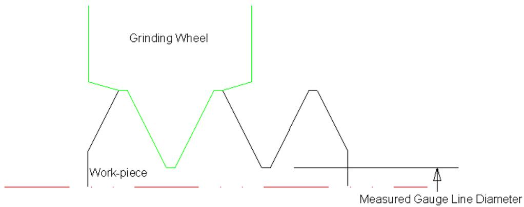
Using the handwheel in X,Z and C, align the formed grinding wheel to the pre-cut component.
