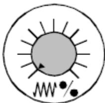
This rotary switch allows you to proportionally control the programmed machine axis speed during automatic cycle operation.
