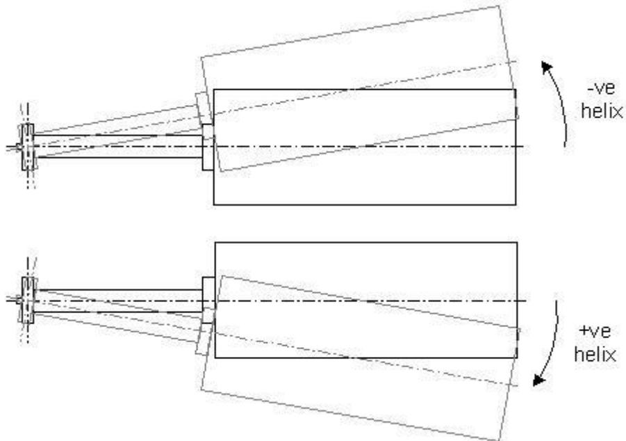
The sketches above show the direction of the spindle helix setting angle as viewed from the front of the machine.
