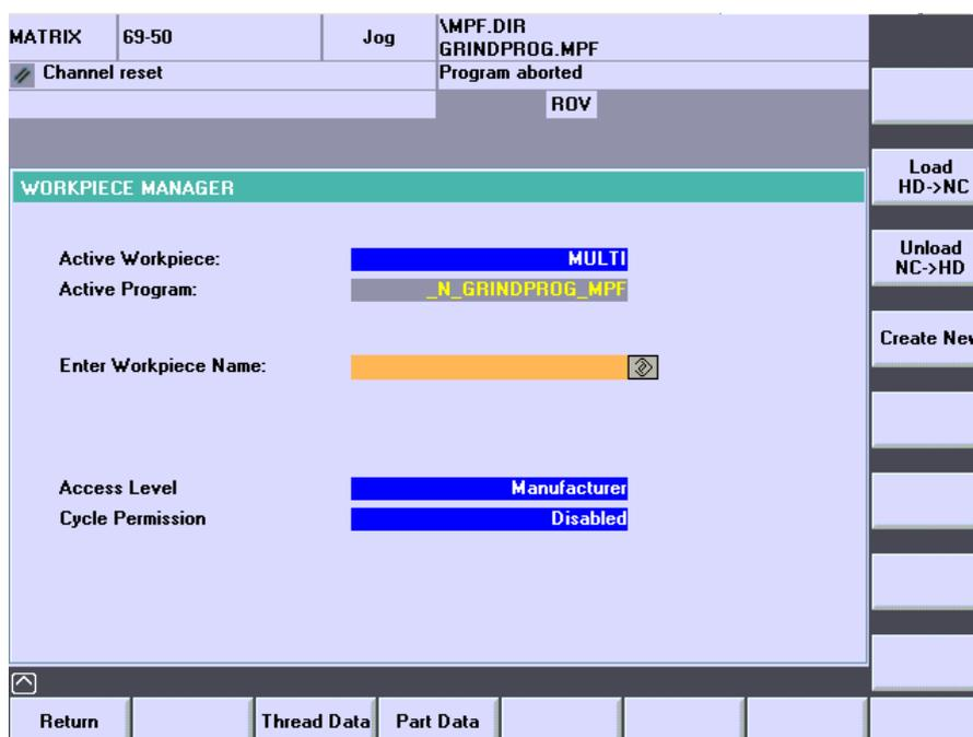
4. Enter a name (max 8 of characters) for a workpiece that you want to grind in the Enter Workpiece Name input field followed by pressing the yellow [INPUT] key on the HMI panel.
