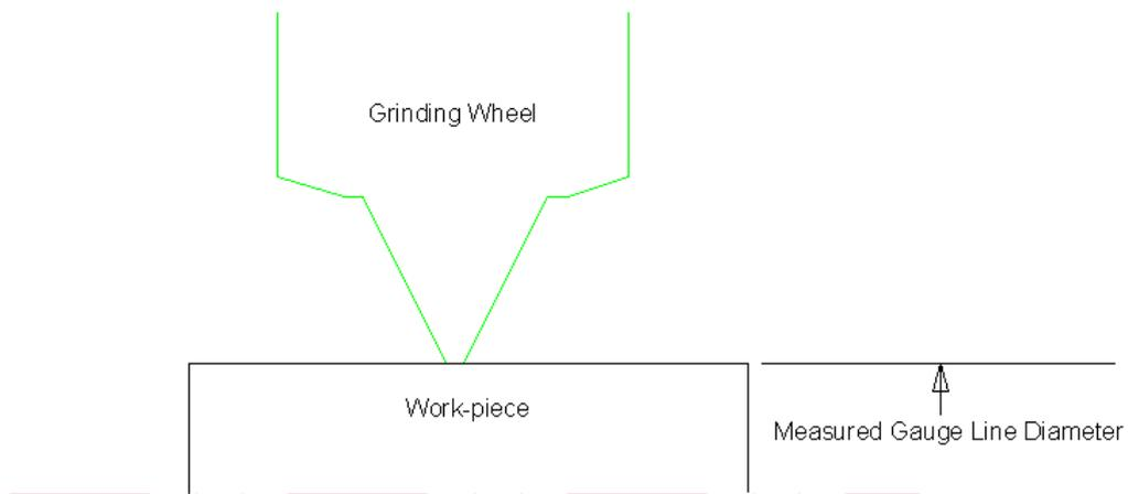
Using the handwheel in X,Z and C, align the tip of grinding wheel to OD of the workpiece.
