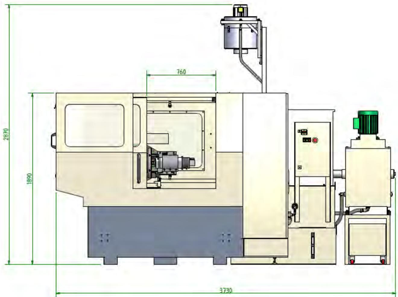
Minimum workshop height where machine is to be installed = 3000mm
