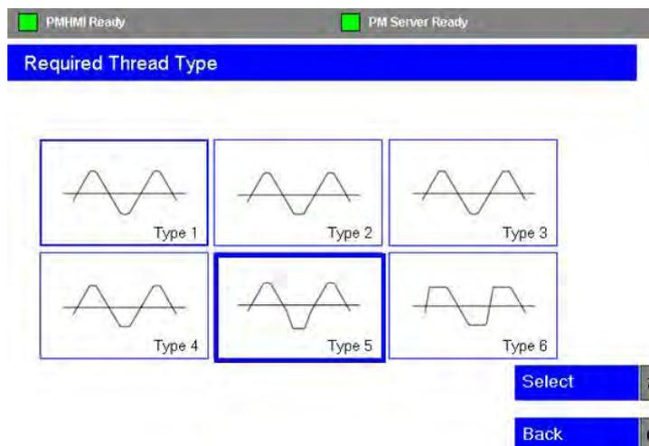
1. Highlight the Type 5 icon using the blue arrow keys on the HMI panel or by using the TAB key.
