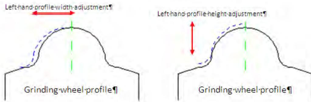
The adjustment is applied at the profile mid-point on completion of the right hand profile and prior to execution of the left hand profile.
