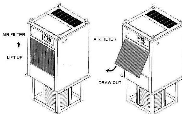
2. Use a vacuum cleaner, compressed air, water and brush to clean the filter. Allow the filter to dry after cleaning before re-assembling. Clean once every 2 weeks with neutral detergent.
