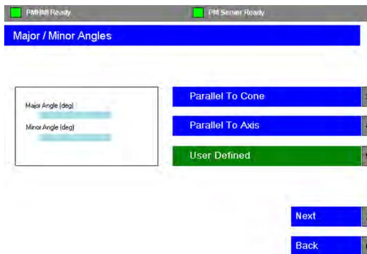
Enter the Major (addendum angle) and Minor (dedendum angle) angle values in the input fields and then select the [Next] softkey to continue. The angle can be specified as a positive or negative value. Fig.3 below shows the affect that positive major/minor angle has on the thread profile.
