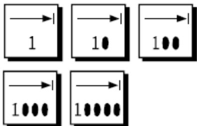
Select to jog the selected axis by a preset incremental amount with each press of the jog [+] or [-] key.
