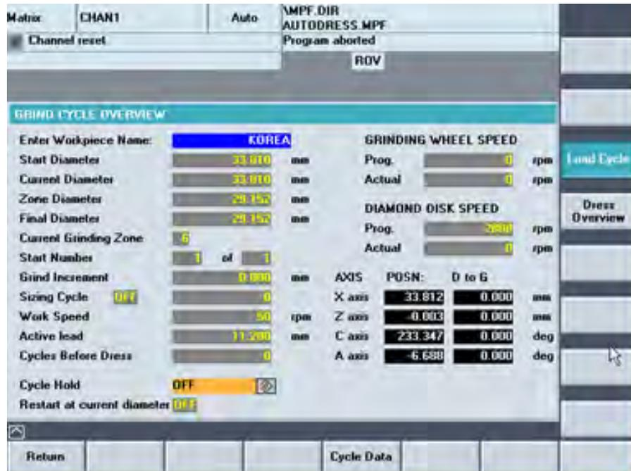
This screen automatically gets updated as grinding progresses through each of the defined grinding zone (G1 – G5).
