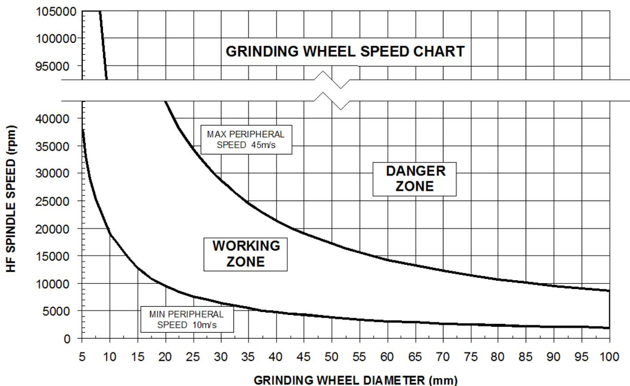
You should ensure that the grinding wheel speed operates within the “Working Zone” shown on the chart.
